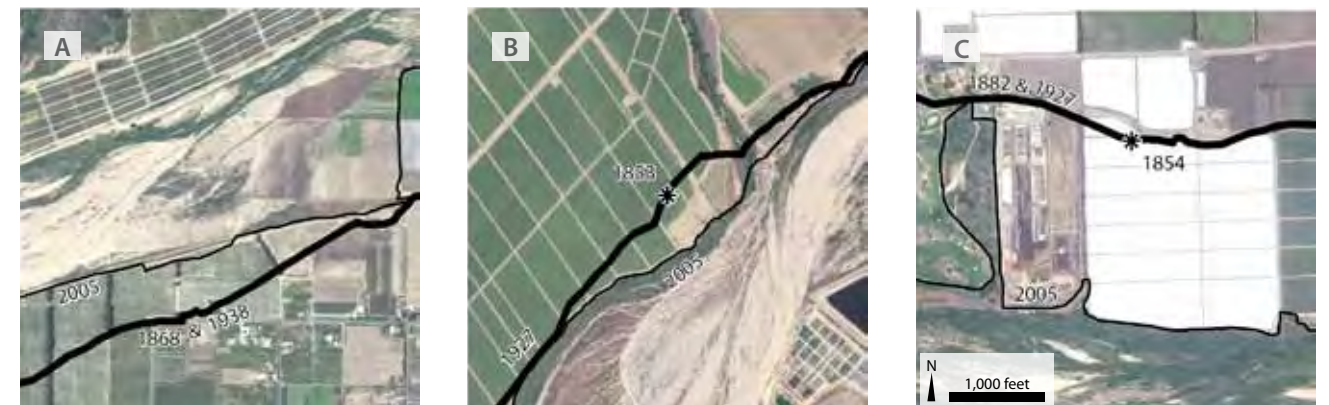
Fig. 3.17. Examples of historical persistence in bank location. In many locations along the river, the position of the outer bank remained quite stable over decades, despite intervening major floods (including the St. Francis Dam break of 1928). This is illustrated here in three reaches: south of the Sespe Creek confluence (left), at South Mountain (middle), and at the Olivas Adobe near the river mouth (right). In each case, early (1854-1882) evidence also confirms the early 20th century (1927-1938) bank position. In each instance, by 2005 bank position has shifted somewhat. (USDA 2009)
