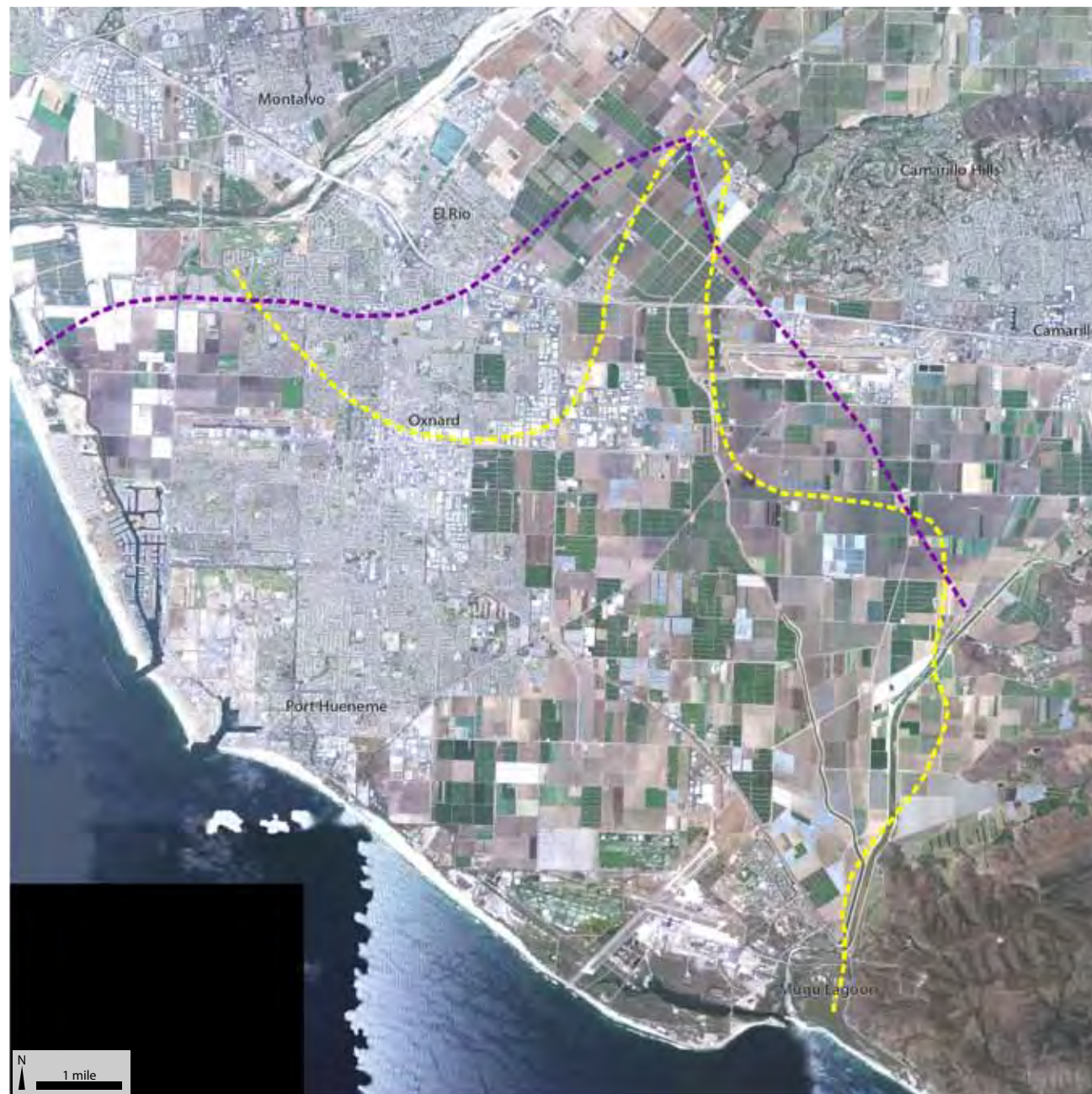
Fig. 5.3. Extent of artesian conditions, 1900 (in purple) and ca.1930 (in yellow). Though both are somewhat coarse delineations, they do suggest some shrinking of the artesian zone in the first quarter of the 20th century. (Schuyler 1900 and Lippincott ca. 1930, courtesy of the Water Resources Collections and Archives)
