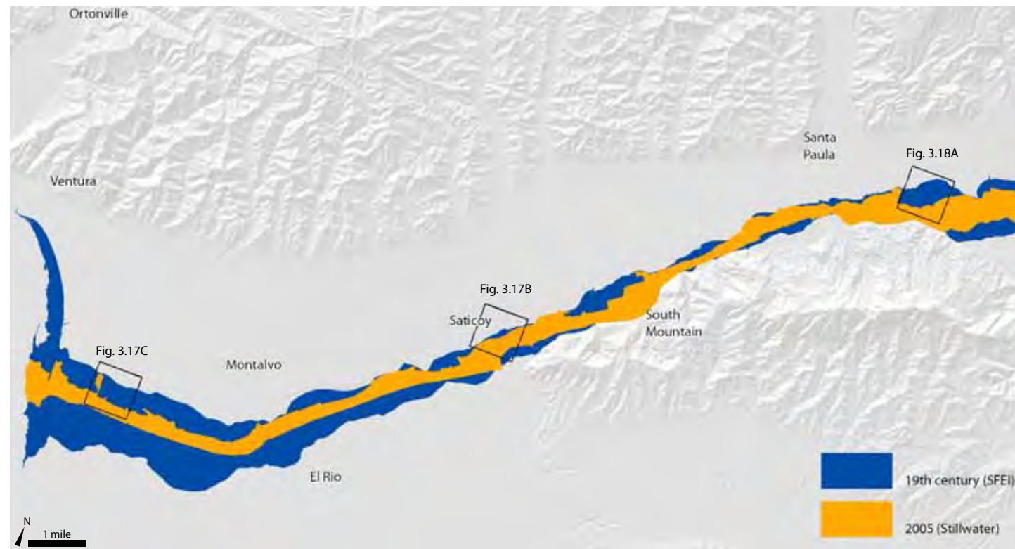
Fig. 3.20. (bottom) River corridor extent and outer bank position, 19th century and 2005. By 2005, over 7,600 acres had been lost, 49 % of the original river corridor area. Much of the lost area was bottomland habitats, leveed and reclaimed for farming and other land uses. Documented change is concentrated particularly in the Oxnard and Estuarine reaches (below Saticoy) and between Santa Paula and Sespe creeks. (2005 mapping from Stillwater Sciences 2007b)
